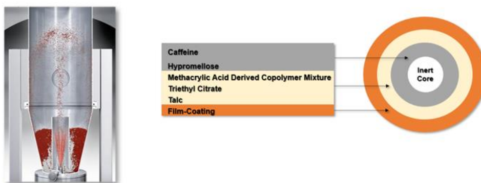
Figure 1. A representative illustration of the fluid bed coater with a Wurster tube (left), and the layers of the pulsatile-release caffeine formulation (right).
